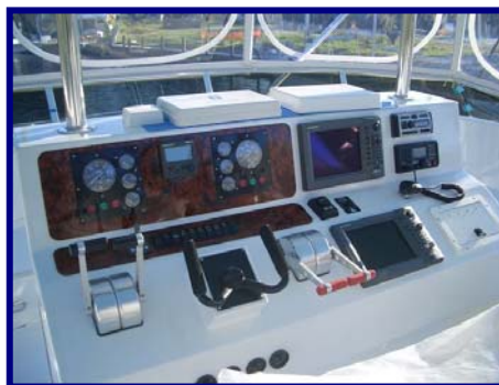
New Flybridge Helm Station
